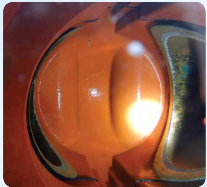
An under-pressure look of clean valve seat.
